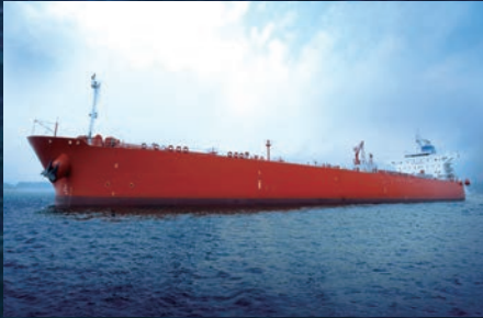
1 320,000 DWT VLCC (Very Large Crude oil Carrier) L x B x D x d : 333.0 x 60.0 x 30.5 x 22.8m Service Speed : 14.8 Knots 2 160,000 DWT CRUDE OIL TANKER L x B x D x d : 274.0 x 49.0 x 23.1 x 17.3m Service Speed : 14.5 Knots
