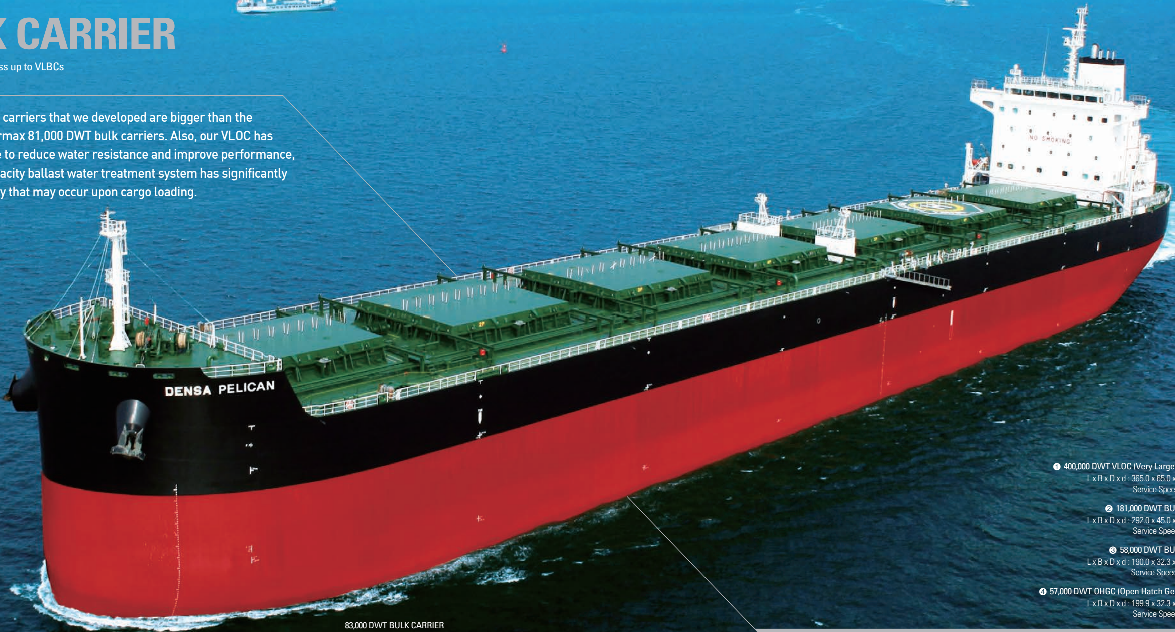
83,000 DWT BULK CARRIER L x B x D x d : 229.0 x 32.2 x 20.2 x 12.2m Service Speed : 14.1 Knots
