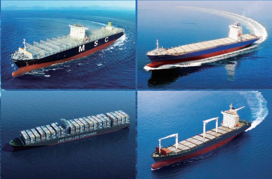
1 13,000 TEU CONTAINER SHIP L x B x D x d : 365.8 x 48.4 x 29.9 x 13.5m Serviced Speed : 25.2 Knots
