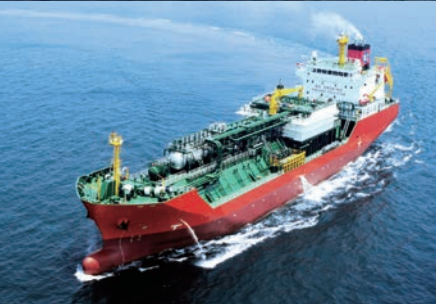
12,000 CBM LEG CARRIER L x B x D x d : 146.2 x 22.6 x 12.1 x 7.4m Cargo containment system : Independent tank, Type C Service Speed : 16.4 Knots
