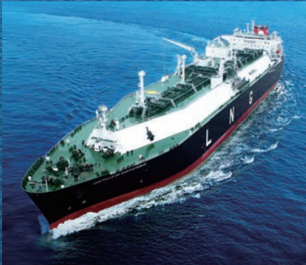
173,600 CBM LNG CARRIER L x B x D x d : 295.9 x 46.4 x 26.5 x 11.5m Cargo containment system : Membrane, NO96 Service Speed : 19.5 Knots
