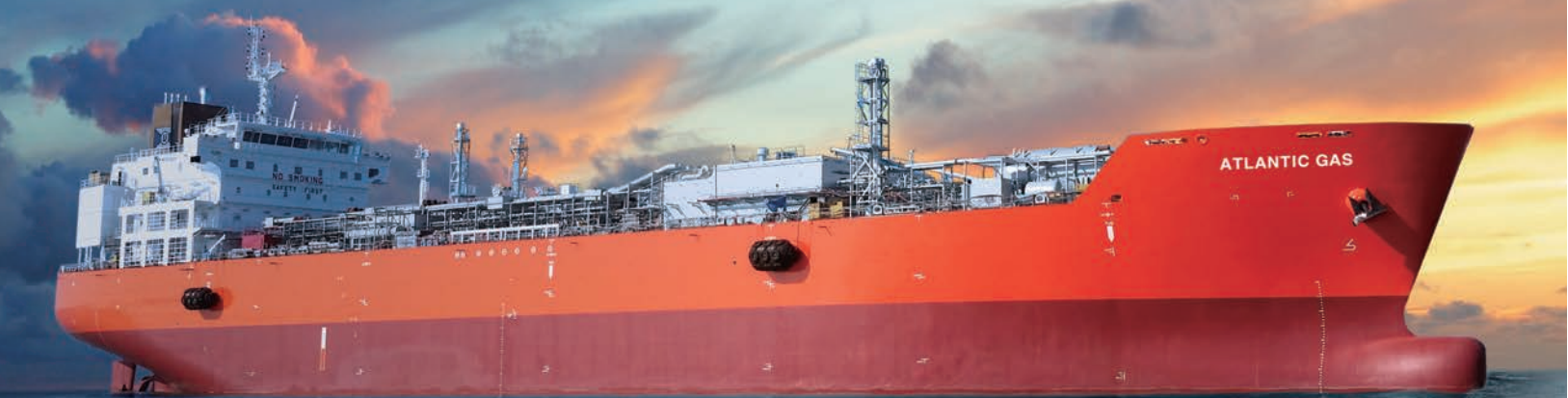
22,000 CBM LPG CARRIER L x B x D x d : 159.7 x 26.6 x 17.4 x 8.4m Cargo containment system : Independent tank, Type C Service Speed : 16.0 Knots
