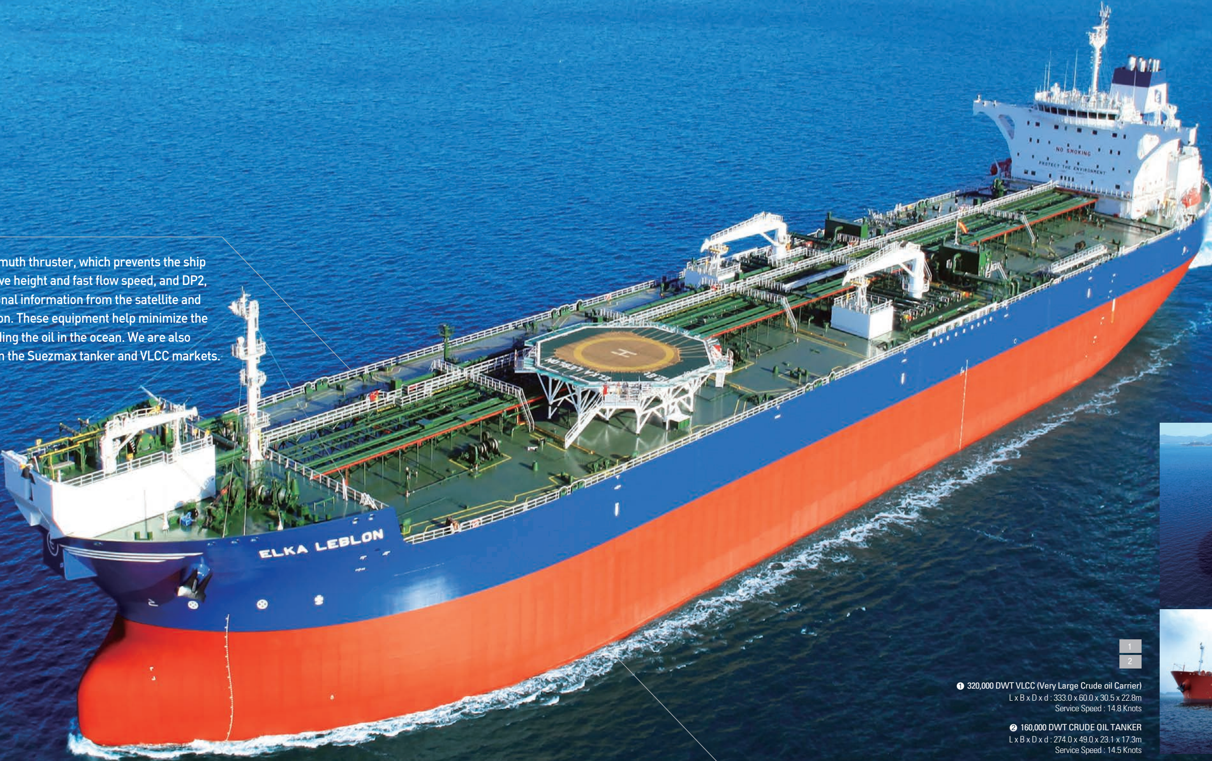
155,000 DWT SHUTTLE TANKER L x B x D x d : 278.3 x 48.7 x 23.6 x 16.6m Service Speed : 15.5 Knots
